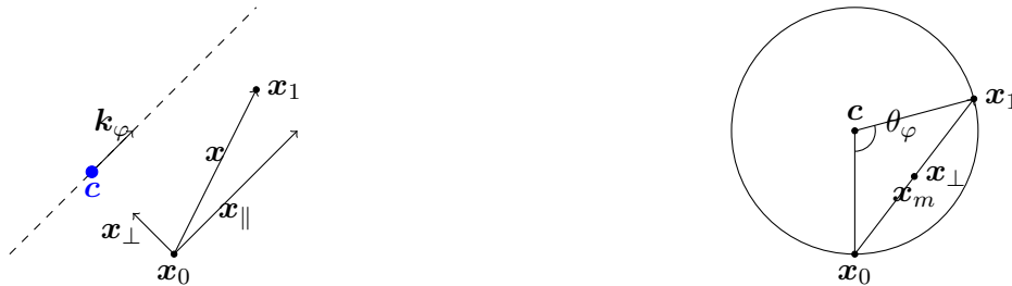
(a) Decomposition of translation into vectors parallel and perpendicular to the axis of rotation \mathbf{k}_\varphi , pictured by the dashed line.
